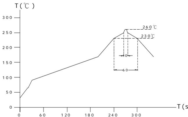
Lead-free the recommended reflow condition
