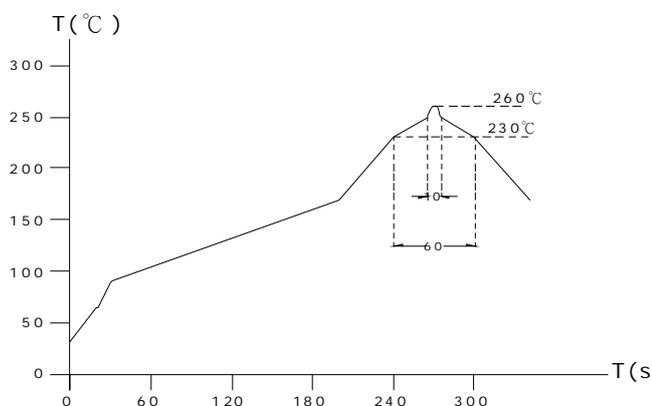
Lead-free the recommended reflow condition
