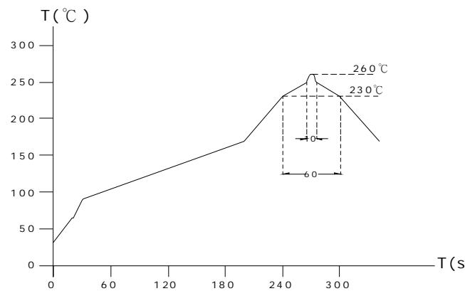
Lead-free the recommended reflow condition
